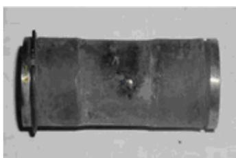
Fig. 1 On-line detection of discharging of suspension potential of plug pin for connection of pulling rod at Phase A of 220kv circuit breaker in XX hydraulic power plant
