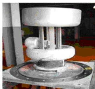
Fig. 6 Failure of insulation pulling-rod discharging in 220kv GIS Phase B circuit breaker of xx power plant
