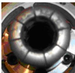
Fig. 3 On-line detection of contact being burnt from reignition of electric arc when 500kv 5013 Phase C circuit breaker is off in xx substation
